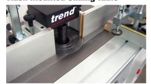
Hard wearing aluminium alloy table runs on high precision bearings to ensure maximum durability. Allows safe machining of end grain work particularly tenoning.
