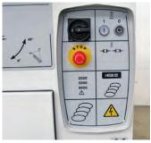
Located on the right hand side of the machine for easy access to all relevant safety buttons and switches. Soft start (automatic star/delta), emergency stop, electrical brake and optional speed indication lights.
