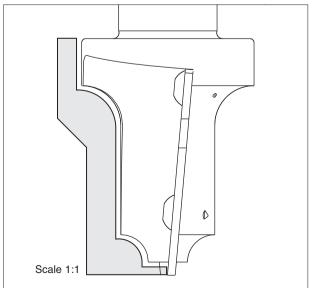
The router bit can be supplied with standard profiles or with knives ground according to customer specification that fit into the shaded area.
