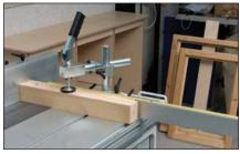
Stops are not required when machining slots and tenons; making errors with the joint production is virtually impossible.
