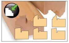
The MWS has 10 alternative moulding profiles including ovolo, lambs tongue,  $9^{\circ}$ ,  $20^{\circ}$  and full splay, making it very versatile.
