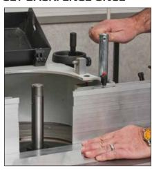
The gauge is placed on the spindle and the backfence is adjusted in line with the outer edge of the setting gauge and then not adjusted again.
