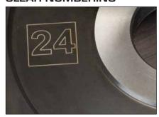
Changing tools takes seconds! Each tool has an individual number for identification to speed up the assembly process for each operation.
