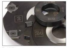
The MWS is easy to use and eliminates costly errors as there are no adjustments needed. All tools and spacers are clearly numbered.
