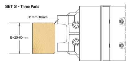
\* Three RH and three LH knives are required for each radius produced.
