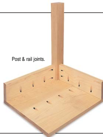
4. Drive self tapping screws to secure.
