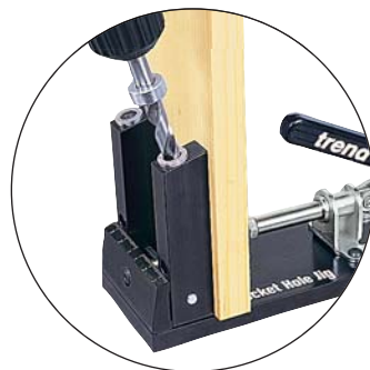
3. Drill pocket hole sockets.
