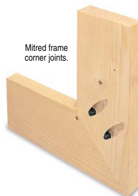
4. Drive self tapping screws to secure.
