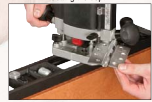
Routing hinge recesses
