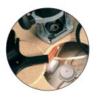
Completed cut When cut, the waste piece is supported by the wings of the jig. The stepped cutter automatically cuts a rebated edge on the waste piece as well as around the edge of the hole.
