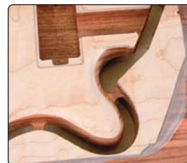
Tags holding mould workpiece in place.
