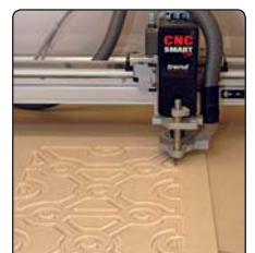
Aperture being cut for glass in kitchen door cabinet.
