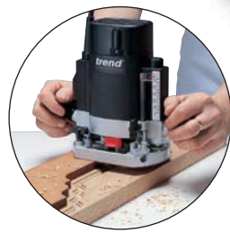
Template guide bush routing
