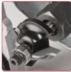
Ogee cutter fitted in a router.
