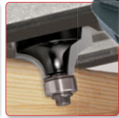
Rounding over a mould.
