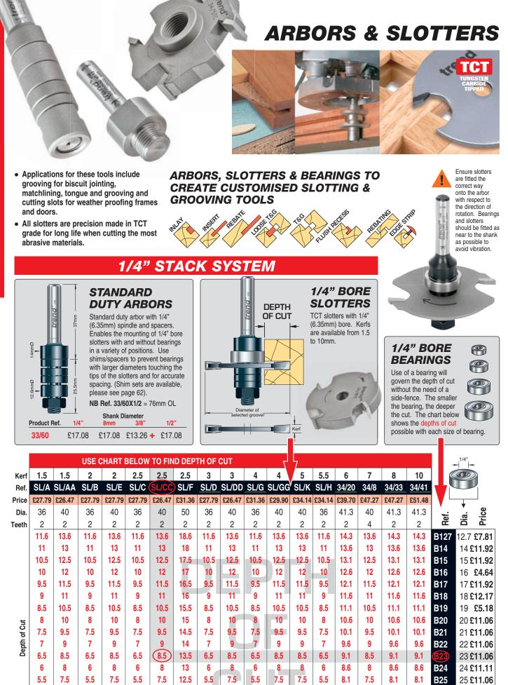
Example - For 2.5mm kerf and 8.5mm depth of cut, choose a 33/60 arbor, SL/CC slotter and B23 bearing.
