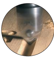
Ref. RT/80 sign engraving in a CNC machine.
