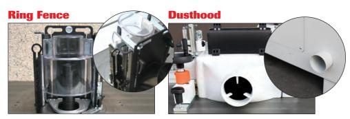
The ring fence comes as standard with the machine and replaces the back-fence when producing curved and circular work. It comes complete with adjustable guarding, lead on finger and a 100mm diameter dust extraction port.
