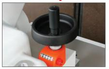
The back-fence has an integral micro-adjuster which controls the position of the complete back-fence.
