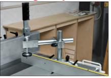
The eccentric clamp comes as standard with the machine and fits into the locating slot on the sliding table. It provides firm and positive clamping, essential when performing any tenoning operation.
