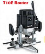
The T10E 1/2" router features a 2000 watt motor with electronic full wave variable speed and soft start, two column precision base, spindle lock for easy cutter changes, micro-adjuster parallel side-fence, precision one-piece multi-slit collet, 3-position revolving depth stop for fast settings and an adjustable inner plate for guide bush accuracy. Includes a 30mm steel guide bush, which is required for the jigs.
