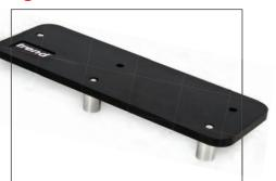
This jig enables any drill to machine the holes in a spelch block for use on a spindle moulder when tenoning. The holes are correctly spaced to suit the M8 holes on the TSM100 tenoning fence and give the correct timber depth to prevent breakout when producing slots and tenons.
