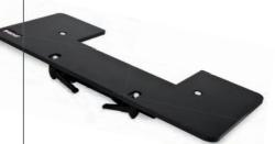
This jig enables any 1/2" capacity router to rout out the pocket in the sliding box sash pulley stiles. Constructed from 10mm solid laminate with integral steel clamp. It clamps to the pulley stile and repeated passes are taken to reach the depth required. The same jig will also rout out a rebate for the pocket to locate into. A 30mm guide bush and 12mm cutter are required.
