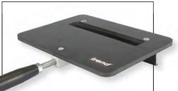
This jig enables any 1/2" capacity router to rout the 12mm slot to accept the Trickle Vent. Constructed from 10mm solid laminate with integral steel clamp. It clamps to the head and repeated passes are taken to reach the depth required. A 30mm guide bush and 12mm cutter are required.
