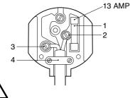
Never use a light socket. Never connect the live (L) or neutral (N) wires to the earth pin marked E or  $\frac{1}{2}$  .
