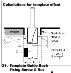
The template guide bush fixing set s and nuts (21) are used to secure the template guide bush (20) to the router base (10).
