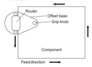
After the edge has been routed, release plunge and switch off router.
