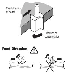
When routing along an edge, the direction of the router travel should be against that of the rotation of the cutter. This will create the correct cutting action and prevent the cutter 'snatching'. It will also pull the router towards the workpiece and hence the side-fence or guide bearing will be less likely to wander from the edge of the workpiece.
