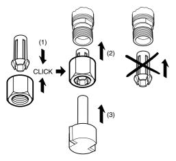
How to Fit and Remove a Router Cutter
