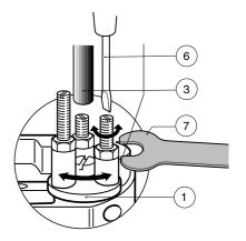
By turning the turret stop, three depth settings can be quickly made.
