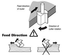
When routing along an edge, the direction of the router travel should be against that of the rotation of the cutter. This will create the correct cutting action and prevent the cutter 'snatching'. It will
