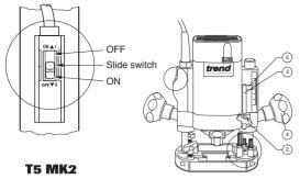
The T5 MK2 router is fitted with an easy reach deadman's switch
