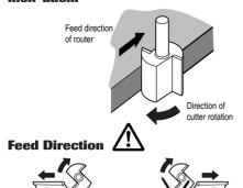
When routing along an edge, the direction of the router travel should be against that of the rotation of the cutter. This will create the correct cutting action and prevent the cutter 'snatching'. It will also pull the router towards the workpiece and hence the side-fence or guide bearing will be less likely to wander from the edge of the workpiece.
