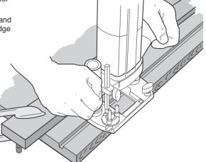
Standard technique is used, and side pressure applied to ensure the router does not wander from the hatten
