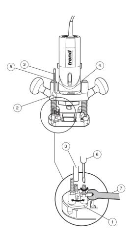
By turning the turret stop, three depth settings can be quickly made.
