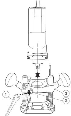
Always unplug the machine from the power supply before separating the router from its plunge base.
