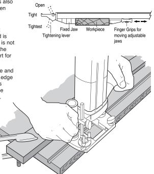
Standard technique is used, and side pressure applied to ensure the router does not wander from the batten.
