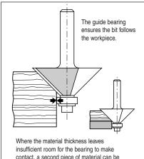
insufficient room for the bearing to make contact, a second piece of material can be temporarily fixed beneath it for the ball bearing to follow.
