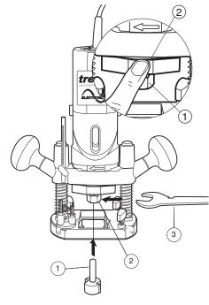
**Correct Sequence for Fitting Collet, Nut, Collet Spring and Bit**
