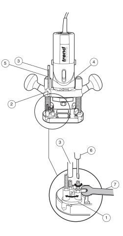
By turning the turret stop, three depth settings can be quickly made.
