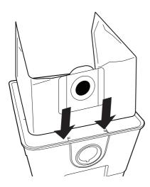
Insert the container hose deflecting bayonet with hose bayonet cap into the inlet and turn clockwise until locked.
