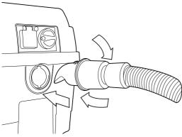
To remove bag undo the container hose deflector with hose bayonet cap by turning anti-clockwise and remove. Slide up collection bag. Close the bag by sliding the tab.
