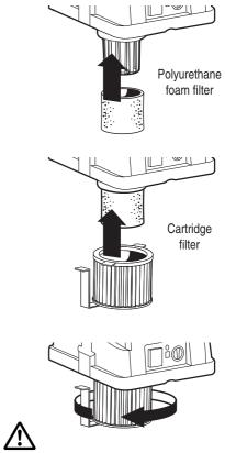
Before using the appliance always check that always check that all the filters provided are in the correct position.
