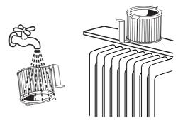
It is recommended however that this filter be replaced every six months, or in relation to the frequency of use and to the type of dirt.
