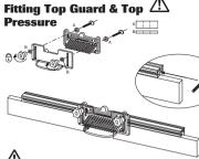
For some applications the thick and thin washer can be swapped over. For example, when profile scribing using a pushblock.
