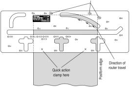
In order to prevent break out of the laminate, rotation of the cutter and feed direction of the router must always be into the postform edge of worktop.
