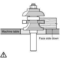
Before using cutter, please ensure it is correctly assembled and locking nut is fully tightened.
