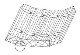
**Curved Joints** – this uses the same technique as the angled joint, but the angles will be shallower ( $5^{\circ}$  to  $15^{\circ}$ ). The overhang will need to be removed as previous.
