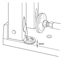
By adjusting the collar back or forward will give a deeper or shallower pocket. If the depth collar
