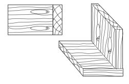
**T- Joints** – faster and stronger than dowel and biscuits. Self clamping whilst glue is drying.
