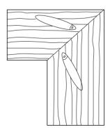
**Square Corner Joints** – faster and stronger than dowel and biscuits. Self clamping whilst glue is drying.
