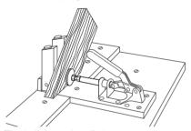
The built-in push-pull clamp arrangement allows both hands to be free for drilling in both applications.
