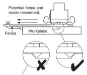
Fence movement will cause cutter to rip into the workpiece.
