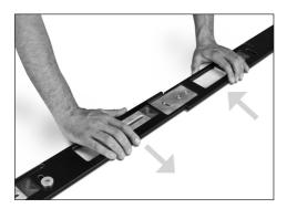
Put two plastic spacers onto each bradawl blade. Take care of the sharp point. When using bradawls always ensure the two spacers are fitted.
