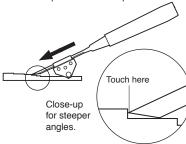
For shallow angles the step is used as a sight line and not as a stop. Look down vertically on the blade and slide blade forward until the end of the blade is in line parallel with the sight line.
