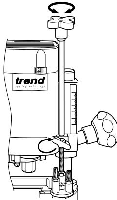
3. Fit cutter into collet.
