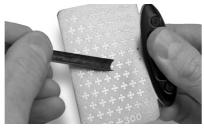
Keep the bevel on the back of the gouge flat on the diamond stone.
