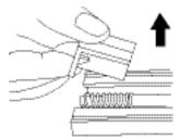
Clip must be positioned as shown during reassembly.
