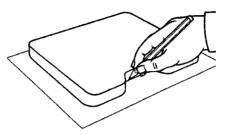
Lay out your router cutters and tools within traced area on paper. Trace, or mark key points and link to produce accurate outlines of your cutters planned out in their desired positions.
