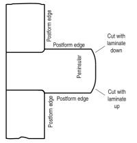
In order to prevent break out of the laminate, rotation of the cutter and feed direction of the router must always be into the postform edge of worktop.
