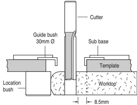
Location bushes are held in position by 'O' rings. Insert the smallest end of the bush into the hole by lightly pushing and turning at the same time. If the bushes are tight use a lubricant on the 'O' ring. Ensure bushes are fully home before use. When using jig ensure location bushes do not foul workbench.
