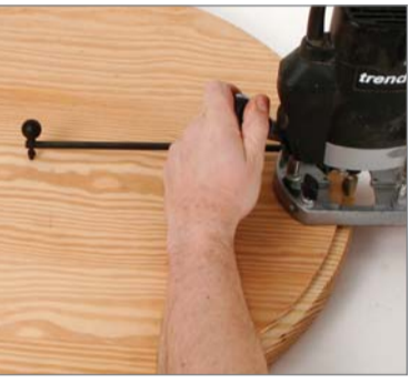
Cut complete circles or arcs with a beam trammel.
