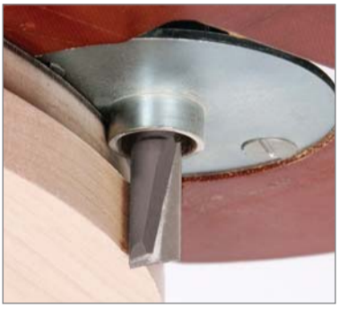
Use guide bushes and templates to create a perfect repeatable shaped or cut out. For straight or shaped work.
