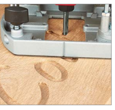
and freehand routing of nameplates.
