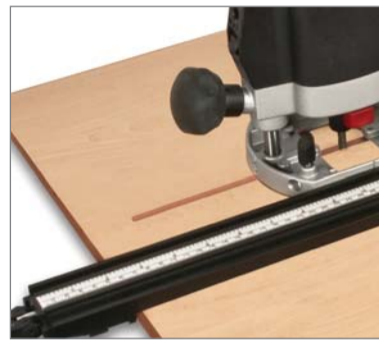
When used portably a batten or clamp guide can be followed with the side of the router.
