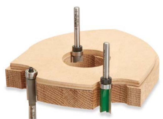
Bearing guided profilers and trimmers can be used to shape the workpiece to replicate exactly the shape of a template.
