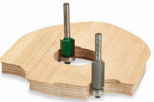
Bearing guided trimmers can be used to trim the veneer using the workpiece as the guide.
