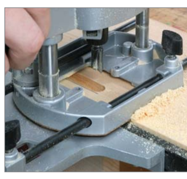
Create rebates, grooves or stopped housings with a side-fence,
