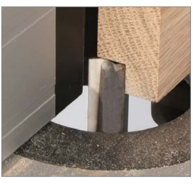
grooving, rebating and full edge profile planing in router tables with the backfence,
