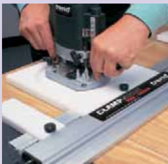
Fitted with the sliding base plate the Pro Track ensures accuracy when routing long lengths.
