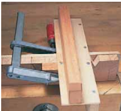
To cut the marble run arches accurately, make up a simple jig to support the router and guide it at right angle across the timber.
