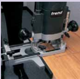
Use the side-fence when cutting recesses parallel to the edge of the workpiece.
