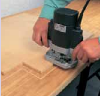
Internal and external templates are used when repeating inlay recess patterns on a number of similar patterns.
