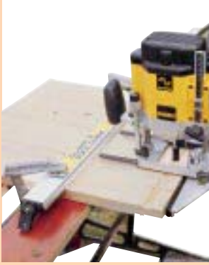
◀ Cutting Rail Tenons
