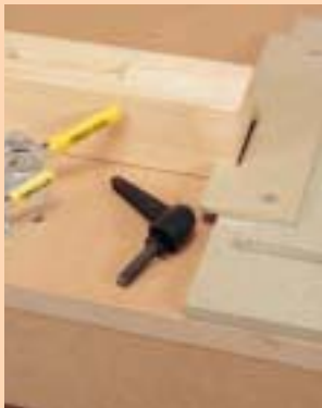
◀ Levers or bolts can be screwed into the threaded inserts to hold jigs and stops
