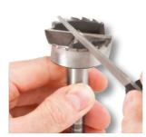
"I PRODUCE A RAZOR SHARP EDGE ON FORSTNER BITS IN SECONDS WHEN UTILIZING THE TREND MINI TAPER FILE."
