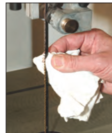
Removes resin & grime from machine bed surfaces
