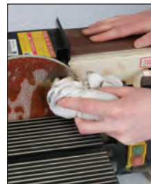
Removes resin & grime from machine bed surfaces
