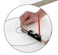
Compass The drawing of circles with various diameters
