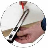
45° Miter Marks a line at 45° to a given straight or flat surface.
