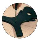
Setting-up The diameter of the finished access hole will be 10". Carefully mark the centre point of the circle, if possible positioning the access hatch between the floor joists. Screw the Routabout jig to the floor using a single No. 8 particle board screw at the centre point to act as a pivot.
