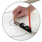
Compass The drawing of circles with various diameters
