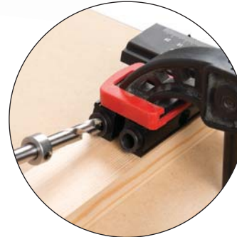
3. Clamp to timber and drill pocket hole sockets.
