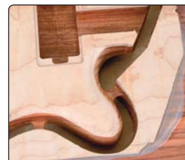
Tags holding mould workpiece in place.
