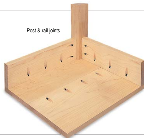
4. Drive self tapping screws to secure.
