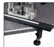
Long pivot clamp securing extrusion to worktop.
