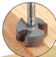
Trimming hardwood lipping with Ref. 37/1.
