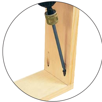
4. Drive self tapping screws to secure.
