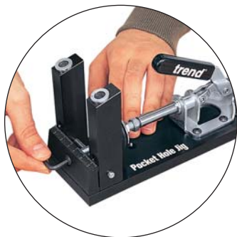
1. Adjust column position.
