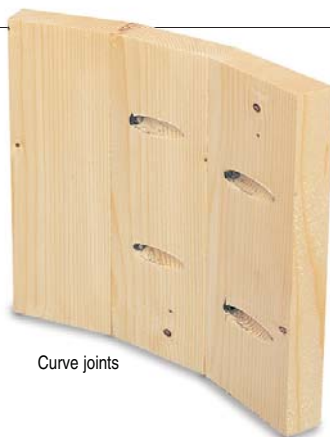
3. Drill pocket hole sockets.
