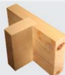
Through housing joint using tenon slide template.
