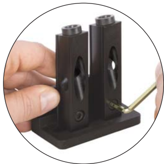
1. Adjust column position.
