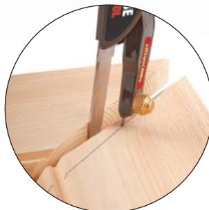
Parallel a cutting line.
