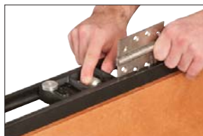
Set the length using hinge as a pattern.
