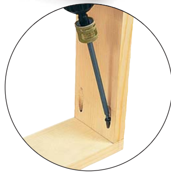
4. Drive self tapping screws to secure.
