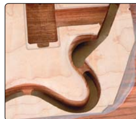
Tags holding mould workpiece in place.
