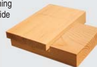
Half lap (halving) joint using tenon slide template.
