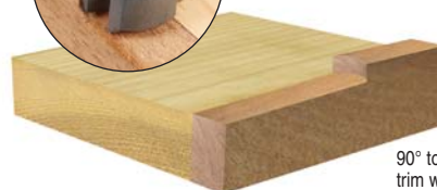
Trimming hardwood lipping with Ref. 37/1.
