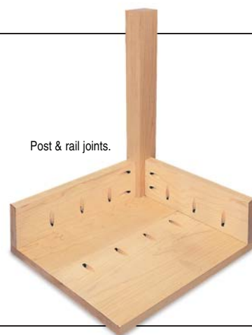
4. Drive self tapping screws to secure.
