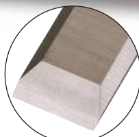
Sharpened at 25° with a razor sharp 30° micro secondary angle.
