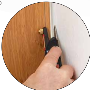
Scribing panels. Lead length can be adjusted. Narrow 0.7mm wide pencil line.
