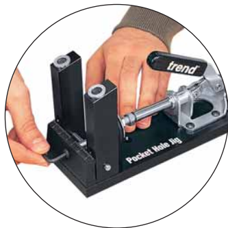
1. Adjust column position.
