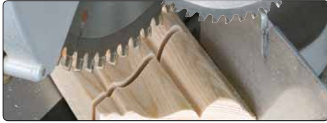
ALTERNATE TOP BEVEL TOOTH FORM
