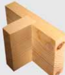
Through housing joint using tenon slide template.
