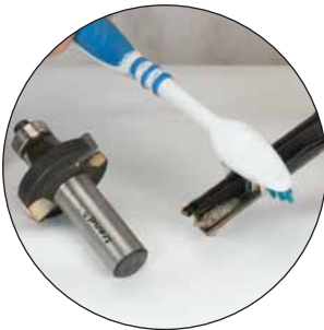
Cleans router cutters.
