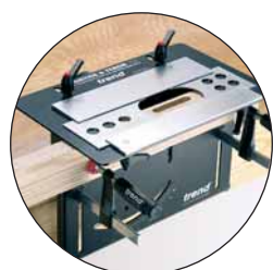
Routing the mortise
