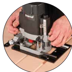
False panel groove copier For creating repeated grooves.
