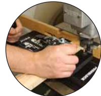
Overhead routing (Guards have been removed for clarity)
