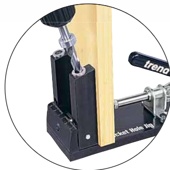
3. Drill pocket hole sockets.
