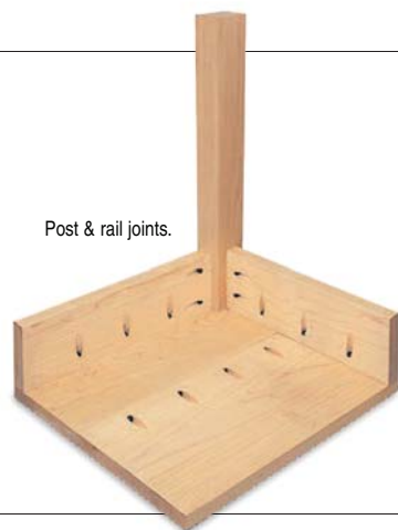
4. Drive self tapping screws to secure.
