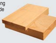
Half lap (halving) joint using tenon slide template.
