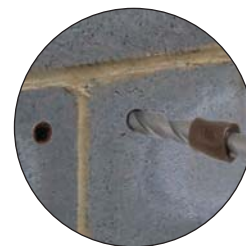
For drilling into building blocks.
