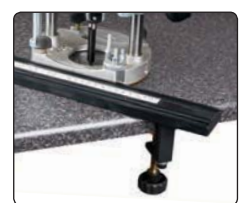
Long pivot clamp securing extrusion to worktop.
