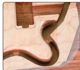
Tags holding mould workpiece in place.
