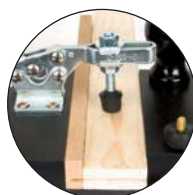
Spelching block facility.
