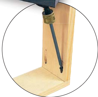
4. Drive self tapping screws to secure.
