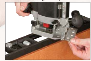
Routing hinge recesses
