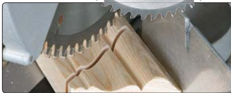
ALTERNATE TOP BEVEL TOOTH FORM
