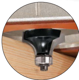
Rounding over a mould.
