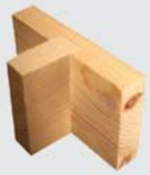
Through housing joint using tenon slide template.
