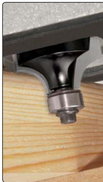
Rounding over a mould.
