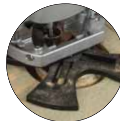
Routing procedure With the guide bush and cutter fitted to the router, place onto the template. The depth is automatically set by a top guide bearing attached to the cutter body. Rotate the router around the centre screw in a clockwise direction, cutting to the full depth in a series of shallow steps until the cutter breaks through.
