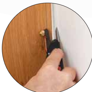
Scribing panels. Lead length can be adjusted. Narrow 0.7mm wide pencil line.
