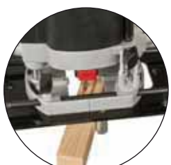
Offset mortising For timber thickness 50mm to 200mm.
