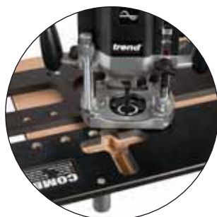
Bolt recess routed.
