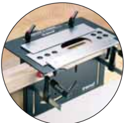
Routing the mortise
