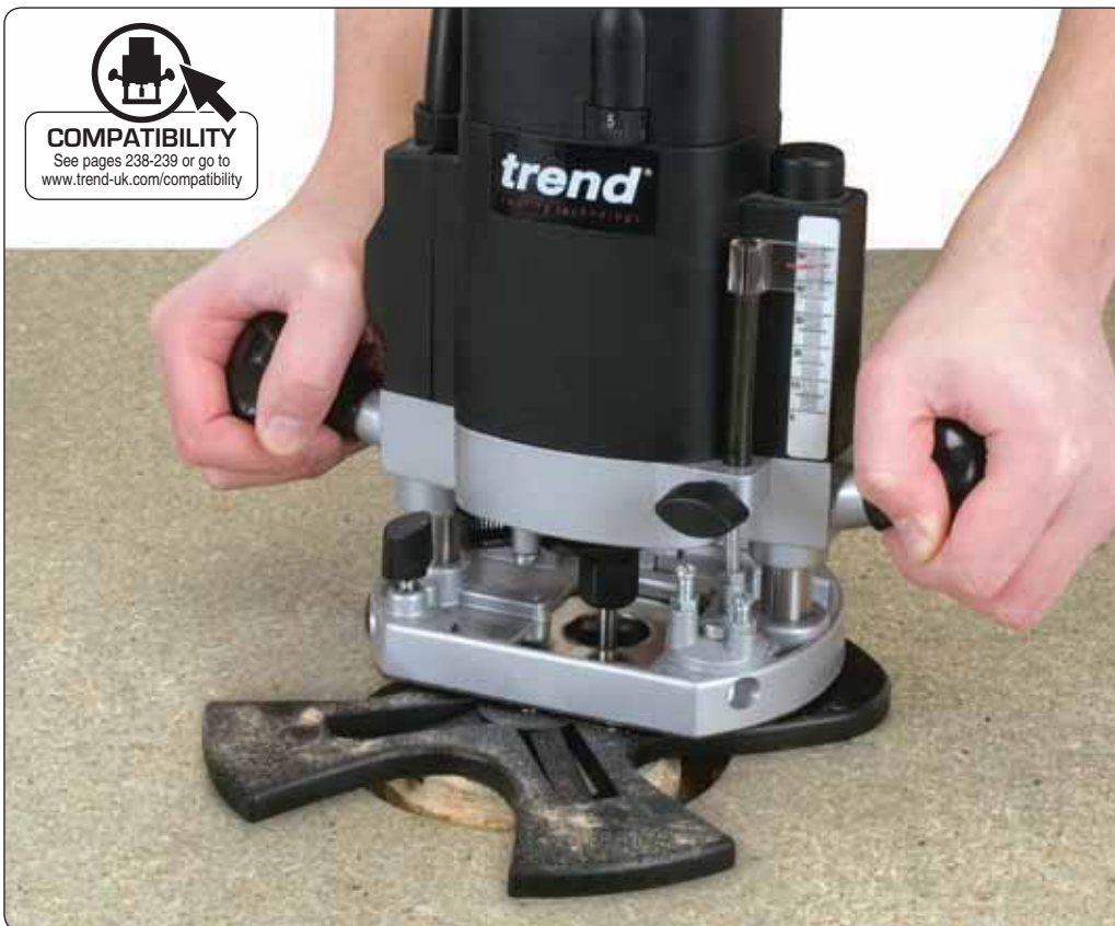
Setting-up The diameter of the finished access hole will be 108mm. Carefully mark the centre point of the circle, if possible positioning the access hatch between the floor joists. Screw the Routabout jig to the floor using a single No.8 particle board screw at the centre point to act as a pivot.
