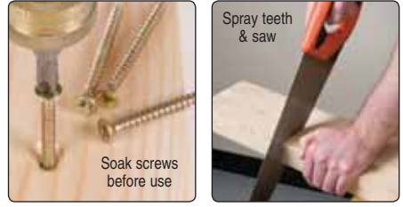
Router Cutter Bearings, Screws and Handsaws Lubricate your bearings to increase tool life. Soak screws for easy driving and keep handsaws in pristine condition to prevent binding.
