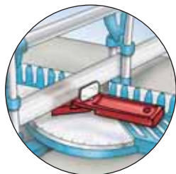
Position the long part parallel to the workpiece and set the sawblade parallel to the metal flag.
